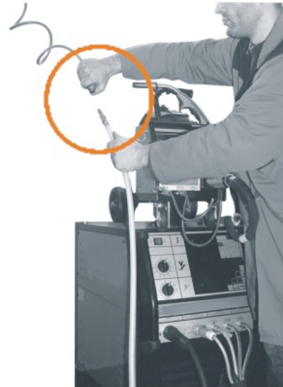
5 - Connect compressed air tube of carbon electrode holder to air supply. Min. pressure 5 bar, min. flow 100 lts/min.
