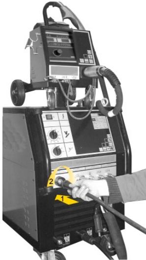
4 - Connect power cable of carbon electrode holder to positive quick plug (+).
