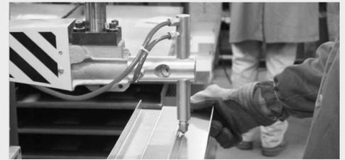
► 50kVA model for automatic cycle sequential welding of steel plates, wires and tubes, stainless steel, zinc, etc., allowing a maximum sequence of 172 cycles per minute. The vertical descent of the upper electrode allows the welding point position to be adjusted correctly.
