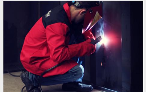
► Pulsed MMA and Liftig pulsed function for lower thermal delivery on thinner plates and greater arc control in the most demanding positions (vertical ascending).
