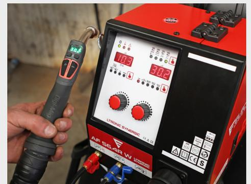
► Electrex DIGIMIG torch option, which includes welding voltage adjustment and reading, wire speed and selection of welding programs visible on the display.
