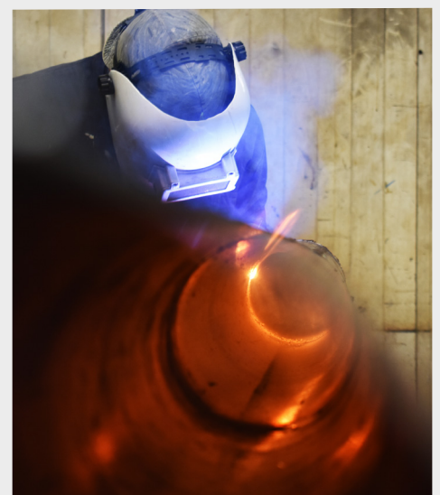
► Electronic inductance adjustment for filling or penetration welds.
