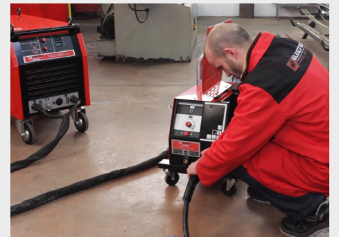
► Possibility of converting the rectifier into a high-performance OPEN-ARC installation without external power with AFFLUX 500.
