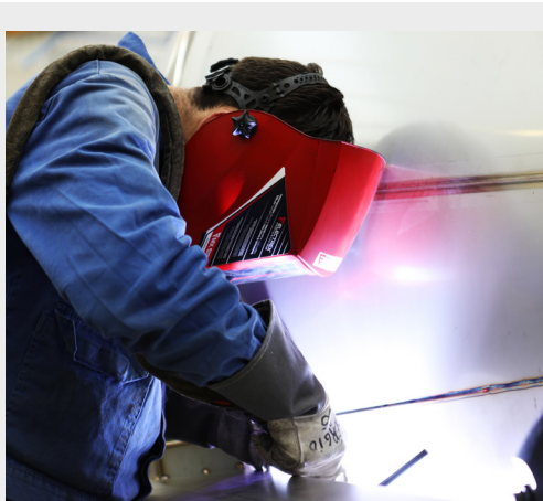
▸ TIG welding with high frequency arc ignition with your rectifier.
